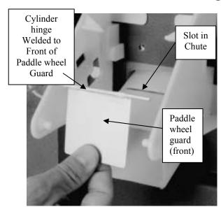
1 When re-assembling the rocking chute/door, the paddle wheel guard is placed in the slot in the ice chute.
